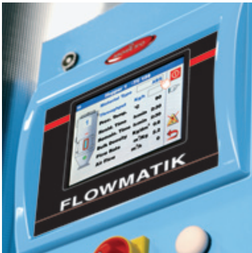
FLOWMATIK control panel equipped with a graphic interface touch screen.
