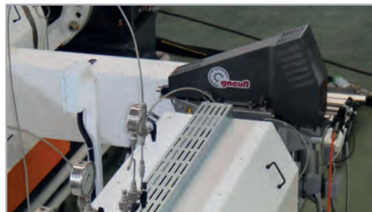
SFXmagnus in the manufacture of foam sheet
